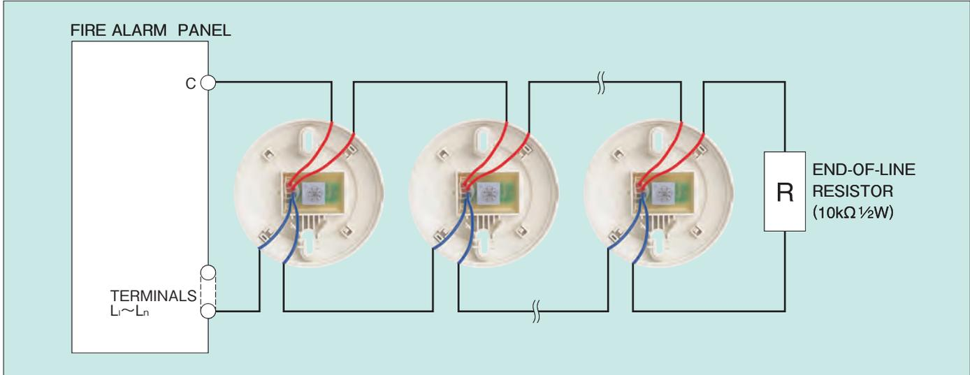
• Lead wire system • Maximum number of detectors to be connected : No limit. • External wire resistance : Less than 50Ω/line
