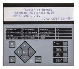
The N765 is equipped with a simple interface and a clear LCD screen to make easy operation possible. The Option button will allow you to change display categories and short cut the function.
