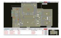
The Windows-based graphic interface application offers the ability of monitoring system conditions of networked fire alarm systems. The system functional button, such as Acknowledge, Signal Silence, Fire Drill, and System Reset, is also available to control networked FAPCs and SMPs.
