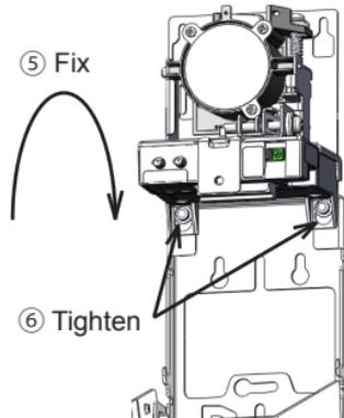
Securely fix the detector to the switch box with four M4 screws
