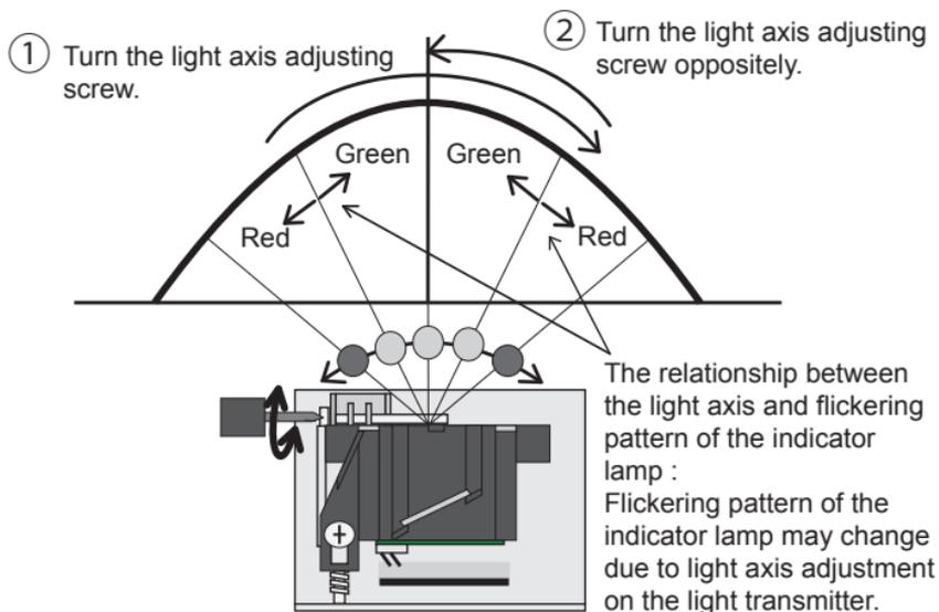
**To ensure stable monitoring of the detector for long period, set the light output to the peak as possible as you can according to the following steps**
