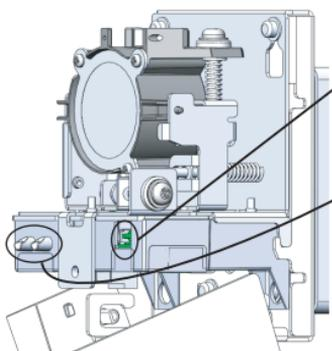
Stand at a position so that you may not **interrupt the light axis** (You can see the detector as shown on the left figure.)
