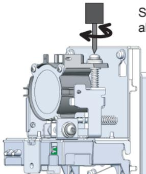
Space for a screwdriver is required in the above of the detector.
