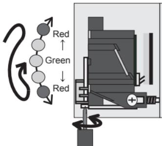
Image of light emission pattern in Horizontal direction (Viewed from the top.)
