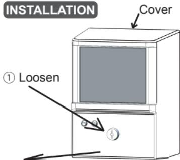
If loosen the cover fixing screw, the cover moves toward you.
