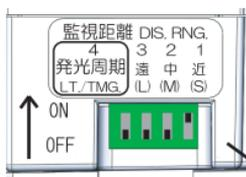
In case of the **light receiver**, set the monitoring range and the light emission cycle.
