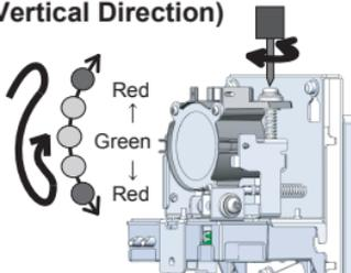
Image of light emission pattern in Vertical direction (Viewed from the side.)
