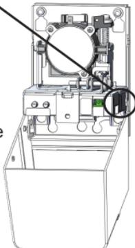
⑨ Remove the body and mount it again to the original position and tighten the two screws.
