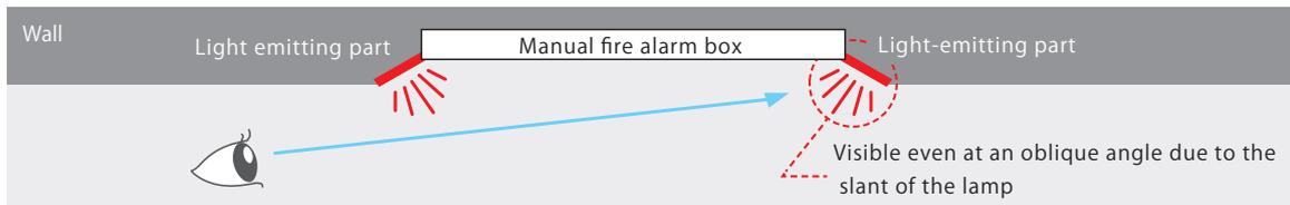
The ring-shaped location lamp positioned around the manual fire alarm box guides you to the exact location of the push button, even in the dark.
