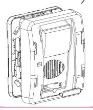
To remove bezel, grip both sides of bezel and pull in a downward and outward motion.
